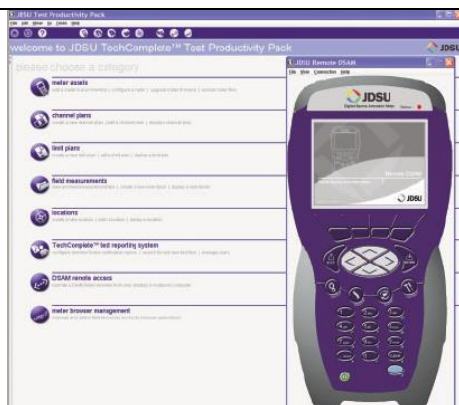
TPP software lets technicians remotely configure, update and upgrade DSAM meters
